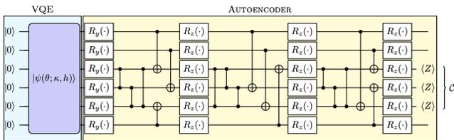
Figure 2: Compression circuit (yellow) and anomaly score measurement ( $\mathcal{C}$ ) of the ground states of  $H(\kappa, h)$  obtained through a VQE (blue). The  $\cdot$  represent independent parameters.
