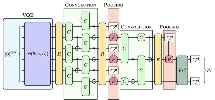
Figure 1: Circuit architecture: VQE states (blue) are the input of the Quantum Convolutional Neural Network composed of free rotations  $R$  (yellow), convolutions  $C$  (light green), pooling  $P$  (red) and a fully connected layer  $F$  (dark green).
