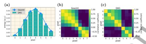
Fig. 6: (a) Visualization of the average calorimeter shower shapes. The energy is given in an arbitrary unit (a.u.) due to image downsampling. The pixel-wise correlation plot for (b) Geant4 and (c) the QAG model. The correlation ranges between -1 and 1; a value of 1 indicates a perfect positive correlation.
