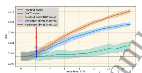
**Fig. 9**: Inference noise study. On the x-axis the noise levels are provided and on the y-axis the MSE as accuracy metrics (the lower, the better). Inference is executed with various noise configurations and on real quantum hardware. At each point, twenty images are generated.
