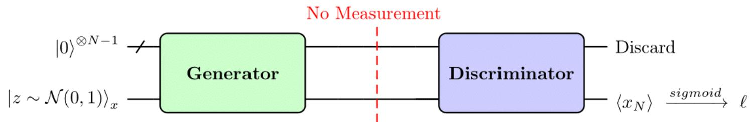
**Fully Quantum model** : Quantum Generator & Quantum Discriminator
